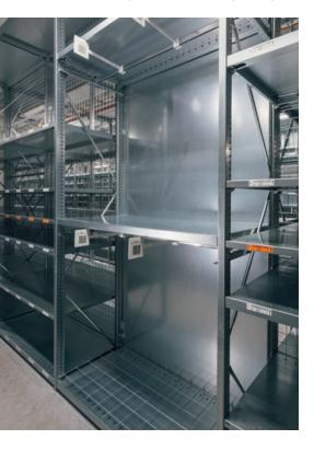
Wire mesh back panel: As an addition to the bracing system, a wire mesh back panel can be installed. This prevents products from falling out the shelving from the back, enhancing extra safety.
