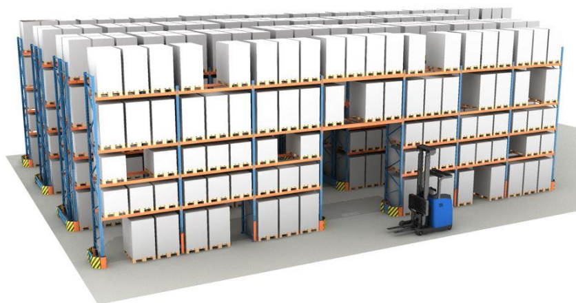
Figure 2: Pallet racking (NR1) with underpass
